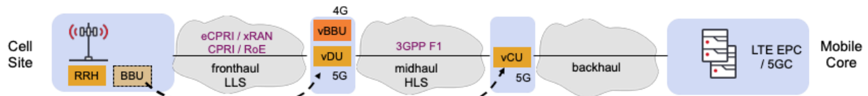
Figure 5.2. Split RAN Architecture.
